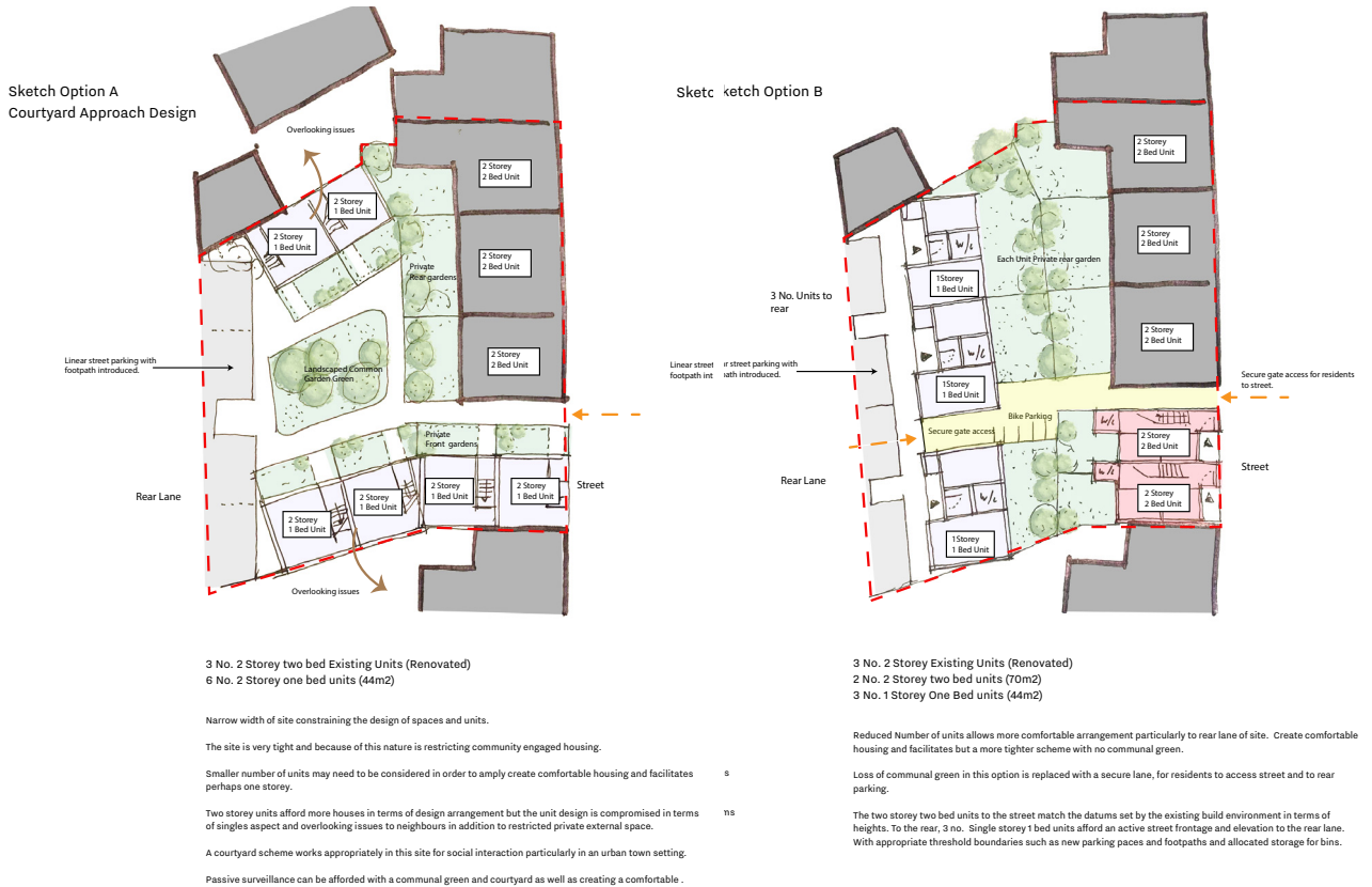
Fig 4.2 Early design concepts by OBFA exploring courtyard and a through lane option
