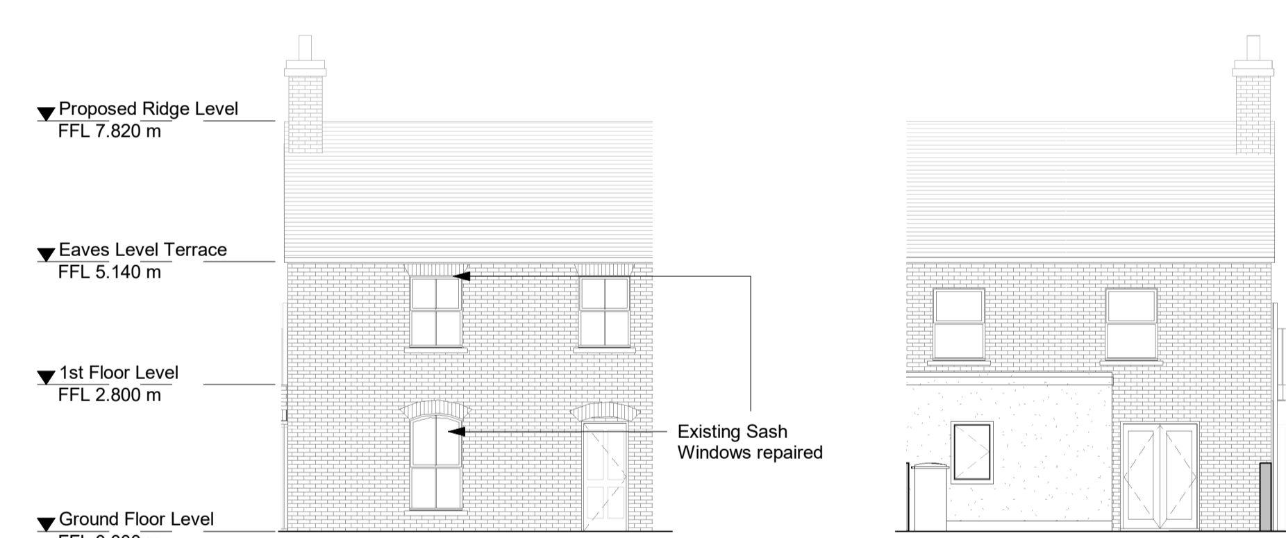
GA_UNIT 3 EAST ELEVATION
