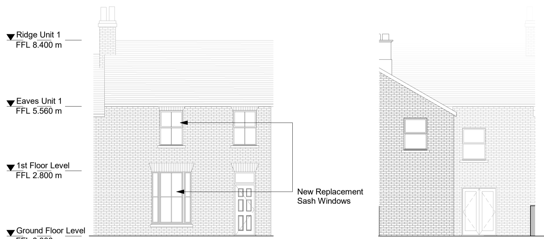
GA_UNIT 1 EAST ELEVATION
