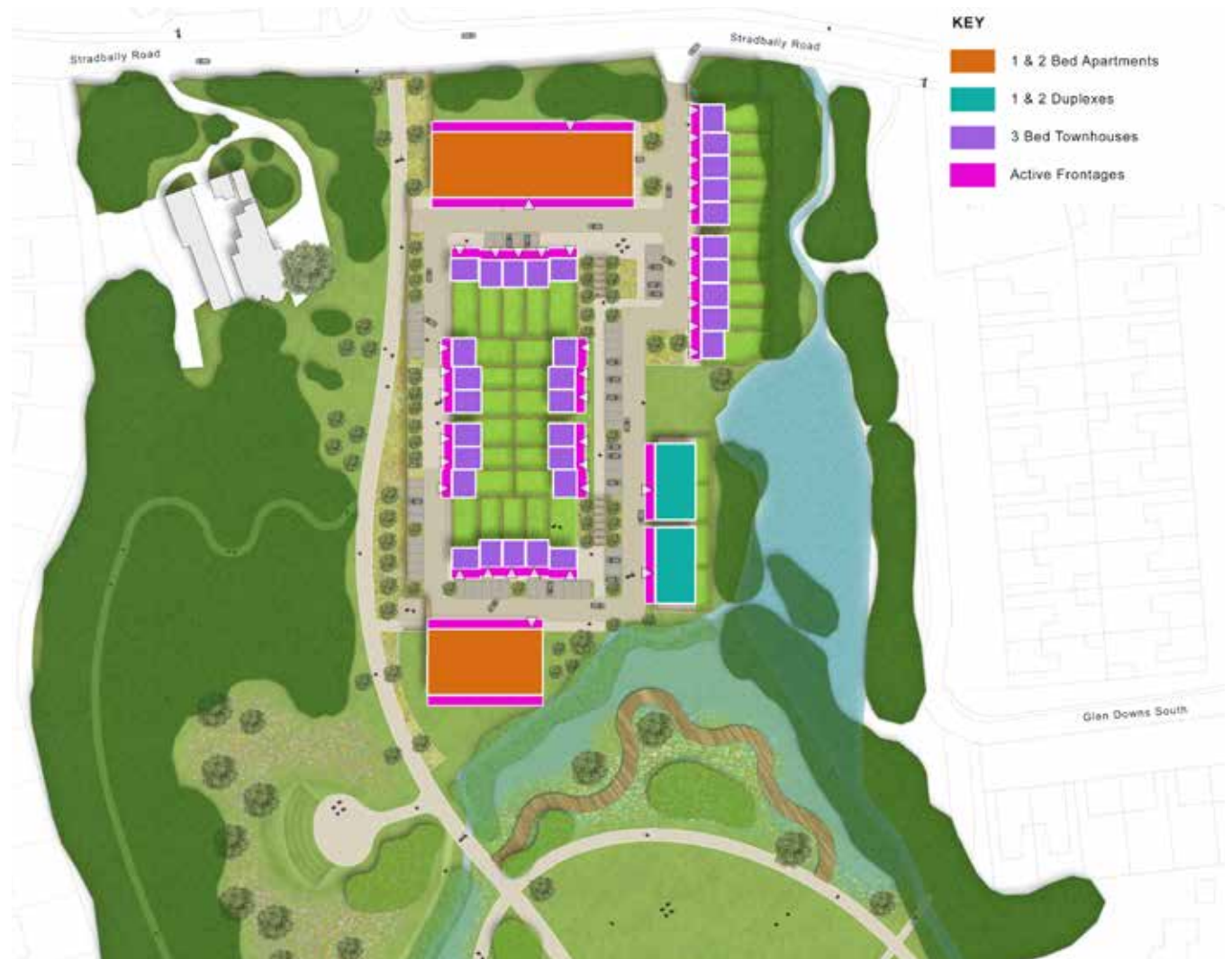
Colour coded masterplan indicating house types, main entrances and views from habitable rooms
