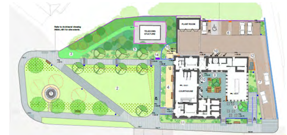
Extract from LGA-L-001 Landscape General Arrangement Plan. Showing the extents of permeable surfacing. All brown and yellow coloured areas is permeable paving and gravel.
