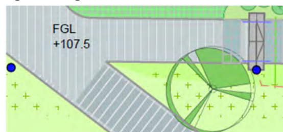
Extract from Landscape General Arrangement Plan. BiO-LGA-001 showing new PCC paving arrangement.
