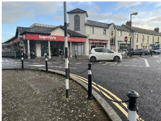
Pedestrian deterrent features
