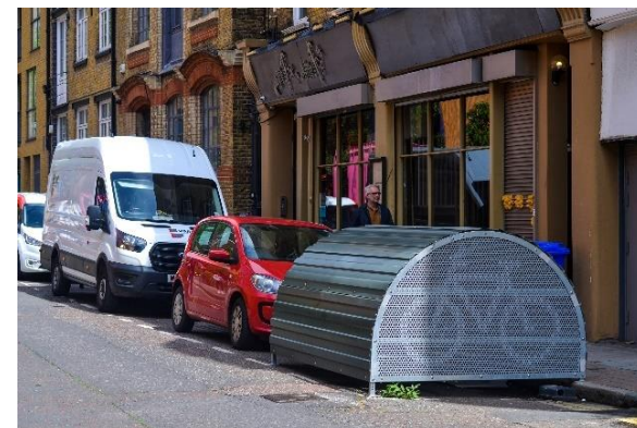
Figure 12-11 Bike hanger on a space previously used for on-street car parking. Hangers provide safe, secure, and sheltered parking for long-stay trips, such as residents of private developments or commuters working in old town centre buildings with no space for bike parking. Photo: DBFL.
